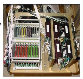
The associated Linux® HIDAS™ interface software provides calibration, diagnostics, engineering unit conversion, and easy-to-use test and checkout of complex I/O. This separates the concerns of the physical hardware from the control and algorithms of the application code.
